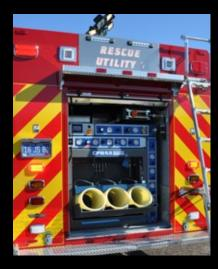
All compressor brands available 13 – 36 CFM with single, double, or triple NFPA compliant fill stations, adjustable shelving, trays, tool boards, electric cable reels, HP breathing air reel, spare SCBA cylinder storage, rehab refrigerator and equipment storage.
