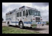
Walk-In Rescue Trucks have all the options of a Heavy Rescue and can be built on Commercial or Custom cab/chassis in body lengths from 12' to 26'. Bodies can be built out of aluminum or stainless steel with walk-in or full walk-through areas with inside storage. Our bodies are available with crew transport style bench seating and up to 78" of headroom to keep personnel comfortable and out of the weather.
