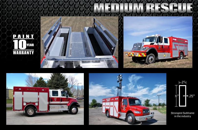
Exterior Options: PTO, Hydraulic or Diesel Generator, Light Towers, Roof Top Storage Compartments with Ladder or Recessed Rear Stair Access, Awnings, Rope Tie-off/Winch Receivers, Front and/or Rear Winch, Trailer Hitch.
