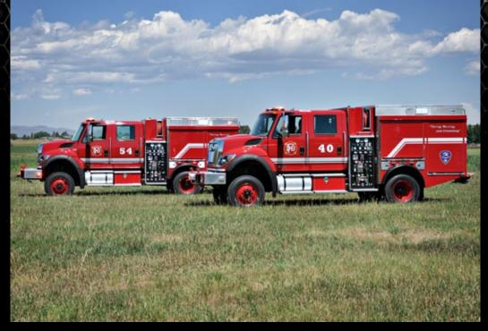
SVI Wildland trucks are built tough to withstand the abuse of offroad fire fighting, built on 4x4 commercial chassis with seating for up to five crew members. The bodies and pump modules are spring loaded for superior strength and available with single and dual pumps from 250-1500gpm, foam systems with CAFs and lifetime guaranteed water tanks from 250-750 gal.
