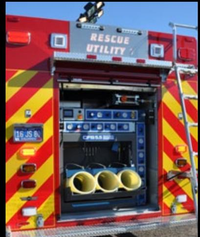
All compressor brands available 13 – 36 CFM with single, double, or triple NFPA compliant fill stations, adjustable shelving, trays, tool boards, electric cable reels, HP breathing air reel, spare SCBA cylinder storage, rehab refrigerator and equipment storage.
