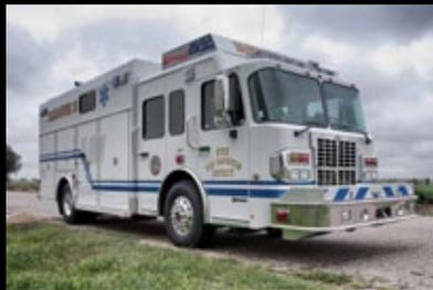
Walk-In Rescue Trucks have all the options of a Heavy Rescue and can be built on Commercial or Custom cab/chassis in body lengths from 12' to 26'. Bodies can be built out of aluminum or stainless steel with walk-in or full walk-through areas with inside storage. Our bodies are available with crew transport style bench seating and up to 78" of headroom to keep personnel comfortable and out of the weather.
