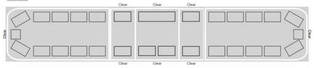
All clear lights {will/shall} shut down when the parking brake is set to comply with "Blocking" mod requirements as outlined in NFPA 1901.
