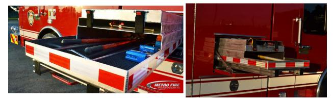
3M<sup>™</sup> Diamond Grade<sup>™</sup> Conspicuity striping shall be provided on the front and side faces of the tray. The striping shall be 2" wide and red/white in color.
