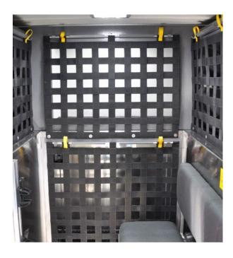
• Cargo netting of 1" - 2" nylon webbing shall be provided over cabinet opening with automotive seatbelt style latches.
