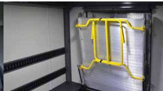
BI-FOLD RAMP FOR EOD ROBOT DEPLOYMENT
