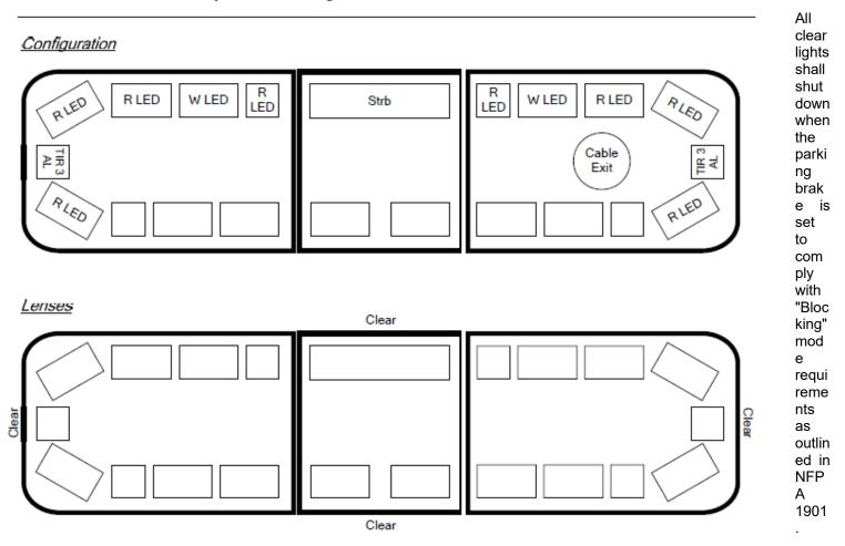
The lightbar(s) shall be separately controlled at multiplex display(s) in the cab.
